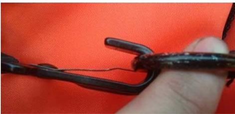
The issue is the spring-loaded tab in the snaphook on the waist belt affecting **some REVERE lifejacket models 198 RT and 160 RT**. The tab has been found to be too long for both the thick or thin design,. When the D-ring of the main waist belt is “hooked,” the length of the tab prevents it from snapping closed. With the hook remaining open, the D-ring is not fully secured. (top photograph) The spring-loaded tab may also lose its resiliency. (bottom photograph)
